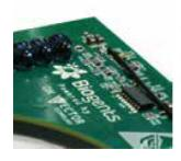
The patented insect sensor consists of arrays of infrared LEDs and light detectors that provide reliable and sensitive detection and differentiation of moquitoes from other objects entering the trap.
