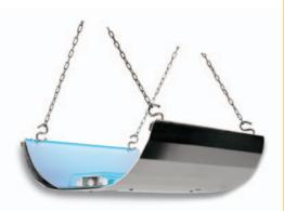
In accordance to HACCP food-processing directive (CE 93/43-96/3-DL 155/97). The special UV-A lamps are set to attract all flying insects to the appliance. When insects approach they remain stuck on the glued paper supplied as a spare part. This appliance allows monitoring and capturing all flying insect within the environment nearby
