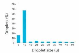
AGROFOG ULV COLD FOGGER alway produces an optimum spray with droplets diameters between 1 and 30 microns. Droplets of less than 10 microns account for more than 70% of the total quantity produced, and those around 20 microns are less than 10%.
